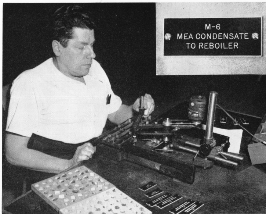
Edmund Matthew of West Machine uses the new tag making machine located in that department. He is shown here making plates for equipment controls. In the upper right hand corner of the picture we find a finished plate.
